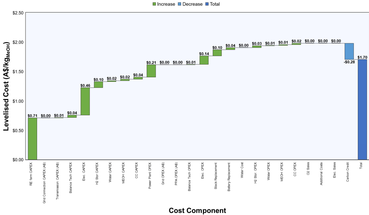
Figure 14: Waterfall plot showing the relative components of the LCOA from sheet 'S2. Results'. NOTE: The values in the figures are for illustrative purposes and will change based on user defined inputs.
