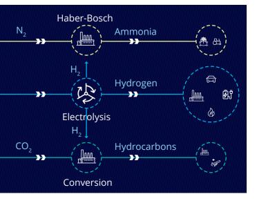
• The substitution of renewable hydrogen with fossil fuel hydrogen in existing Haber-Bosch ammonia plants, will enable a seamless transition to low-carbon ammonia production. This is critical to decarbonising the fertiliser production and industrial explosives sectors, as ammonia is the base feedstock for the industry.
